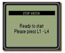
The stop watch screen is the most important screen on UniStop! It is here the timing of the drivers is done. Depending on the number of stop watches running, you will see different layouts of the screen. If you are only timing one driver, you will see more information than if you are timing four drivers!
