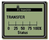
UniStop automatically change to PC mode when a USB cable is inserted. You can't enter PC mode manually.
