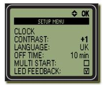
The contrast of the display is the light difference between the dots that are turned on and dots that are turned off. You can manually adjust the contrast setting by selecting "CONTRAST: " and press OK. Then use the arrow up and down buttons to adjust the setting. You can change between –6 and +6. You will see the contrast change at the same time. When the contrast is what you like, press OK again to go back to the setup menu.
