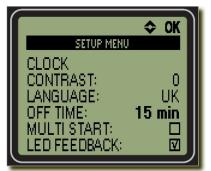
UniStop will automatically turn itself off if it is not used. To save batteries, you want it to turn off as fast as possible, but on the other hand it should not affect the daily work.
