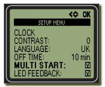
UniStop can start the stop watches in two ways. When Multistart is off, you start each stop watch one at a time. When Multistart is on, you will always start all four stop watches at once. If you want less drivers, you can always use the "REMOVE DRIVER" from the popup menu to remove one.
