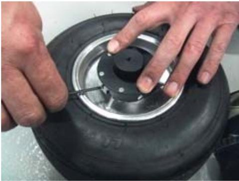
The sensor disc is placed over the centering bush and it is held firmly down. Then tighten the three small screws that fix the sensor disc to the wheel. Tighten the three screws hard, so the sensor disc doesn't go loose when you're driving.
