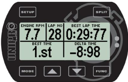
When the Laptimer is passing the finish line, it is showing the difference between the current lap and the best lap and its position. In the shown example, the current lap is 8.98 seconds better than the previous best lap and the current lap is the best lap (in position 1) This information is shown for 5 seconds before changing back to data display. Only times between +/- 9.99 seconds and positions from the 1st to 10th are shown
