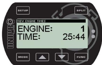
The Laptimer can store the run time of up to 25 different engines, each running up to 999 hours and 59 minutes. Before every training or race, you simply go to setup mode and choose the engine you are using, by using the **▼** and **▲** buttons to find the right engine number.
