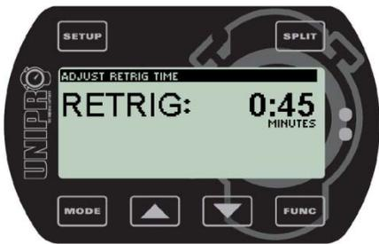
To prevent the problem with IR receivers triggering more than once on a lap, set the Low Delay time to 2-5 second below the normal lap time. When this time is elapsed, the Laptimer turns on power to the IR receiver and enables the trigger again. When the Laptimer is trigged, it is turned off again.
