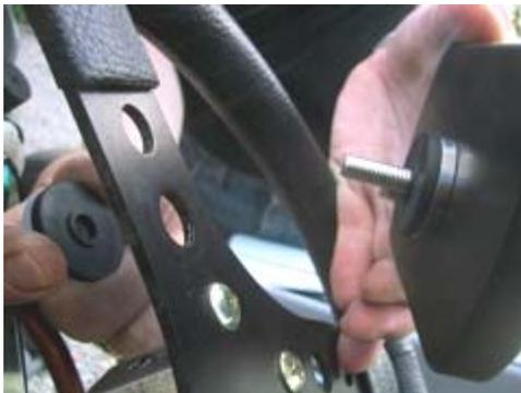
**First, the Display Unit is mounted on the steering wheel.** Choose a hole that gives a good placement at the top of the steering wheel. On some steering wheels, it is necessary to make the hole a little bigger. Remove the nut, the gray washer and *one* of the two black rubber washers. These parts are mounted on the back side of the steering wheel, as shown in figure 1.
