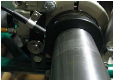
It is also possible to mount the sensor on the rear axle. Also here mount the sensor in the fitting so the distance between the sensor and the sensor disc is between 3 and 10 millimeters
