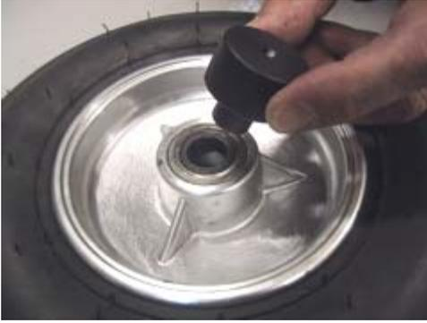
Dismount the wheel and put the centering bush in the inner ring of the bearing. If you drive with front wheel hubs, you must mount the sensor disc on the hub instead of on the wheel – the method is the same as shown here.
