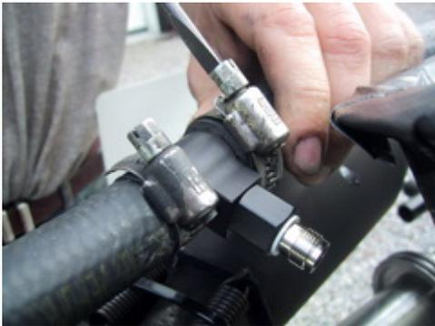
Tighten the two hose clamps to secure the T-junction in the right place.
