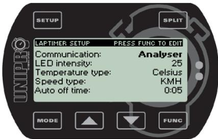
Typical connection to the outside is either IrDA (infrared) or USB. If you set the Laptimer to use IrDA, it will go to PC mode after leaving pit mode. If it is set to use USB, it changes directly to PC mode when the USB cable is connected.
