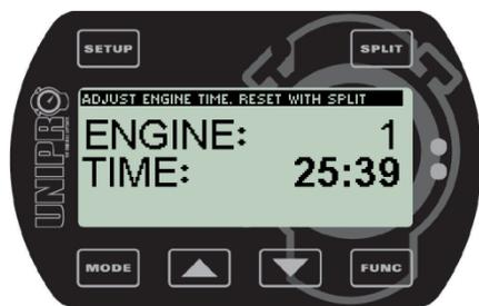
You can use the **▼** and **▲** buttons to change minutes registered on the chosen engine timer. Each press will count one minute up or down. You can press **SPLIT** to reset the timer. Close engine time edit by pressing **FUNC**.
