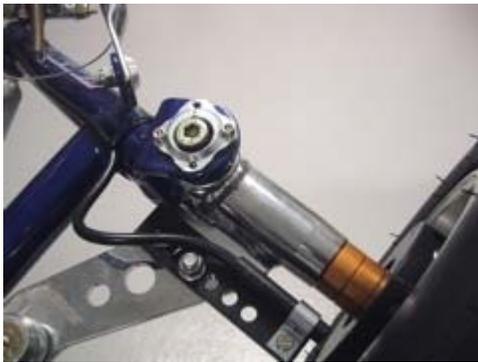
The cable is fixed to the frame in a nice large curve so the wheel can turn without the cable being caught or tightened.
