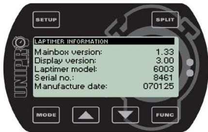
On the Laptimer information screen, you can see the mainbox version, the display version, the Laptimer model, the serial number and the manufacturing date.
