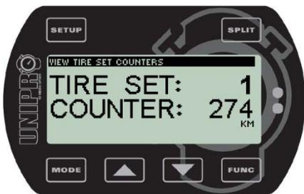
The Laptimer can store the kilometres or miles of up to 8 different sets of tire, each running up to 999 kilometres (or miles).
