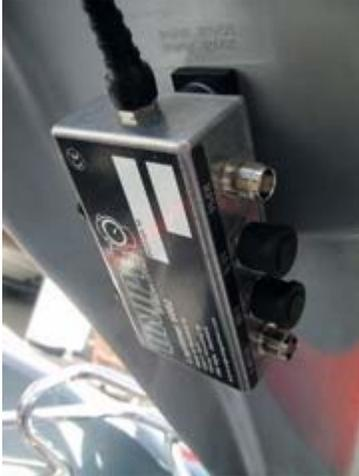
**Make sure that the cable for the Display Unit is pointing upwards.**
