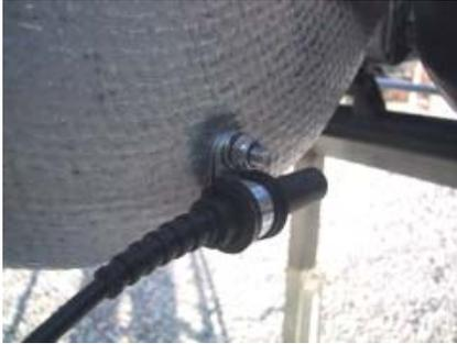
The Loop receiver is mounted parallel with the seat and needs to point backwards against the rear axle. Make sure, that nothing comes between the receiver and the track.
