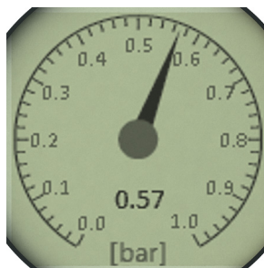
Analog view with 1 bar chosen as max range, and a current pressure of 0.57 bar.
