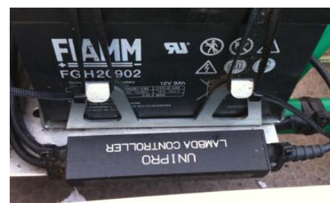
Mount the Lambda controller near the battery.
