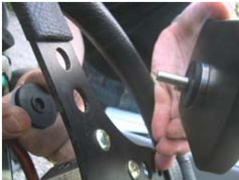
Figure 1. Display unit mounted on steering wheel
