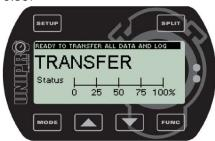
If the Laptimer is set to use USB, you will see this screen when the USB cable is connected. This shows the status of the USB link (PC icon on when USB cable is in) and after this you will choose Receive from the PC Analyser program to start the transmission. When the display shows "Finished" the transmission is finished.
