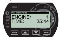
The Laptimer can store the run time of up to 25 different engines, each running up to 999 hours and 59 minutes. Before every training or race, you simply go to setup mode and choose the engine you are using, by using the buttons to find the right engine number.
