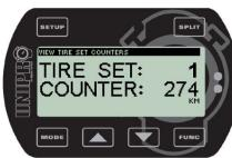
The Laptimer can store the kilometres or miles of up to 8 different sets of tire, each running up to 999 kilometres (or miles).
