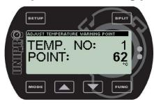
Here you can define a warning point for each active temperature senson. The picture shows the setting of temperature point 1. Use the and buttons to adjust the temperature point. Temperatures are shown in either degrees centigrade or Fahrenheit. If you has activated more than one temperature sensor, you will go to the next warning point by pressing
