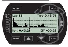
On this screen you can scroll through the laps and see the current lap time, best lap time and the difference between the current and the best lap time well as laps. Together with the numbers there is a graphical view of the difference
