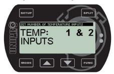
It is here you define how many temperature inputs you are using. Choose the right combination of the 3 temperature inputs. The reason to turn the inputs on or off is to save battery power and to adjust the user interface to the real setup.
