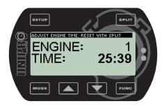
You can use the and buttons to change minutes registered on the chosen engine timer. Each press will count one minute up or down. You can press sput to reset the timer. Close engine time edit by pressing func.
