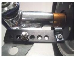
The sensor fitting is mounted in a suitable hole in the stub axle. Depending on the kart model, it can be necessary to drill a hole in the stub axle.
