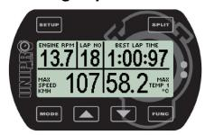
Turning the Laptimer on is done with the button. During power-on, the display will turn on all segments and the 5 LEDs will blink to show start-up is in progress.
