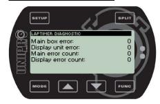
The Laptimer diagnostic screen has mainly information for service purpose. It will show the last error codes for errors from the main box and the display unit, and will show the total number of errors from the main box and the display unit.
