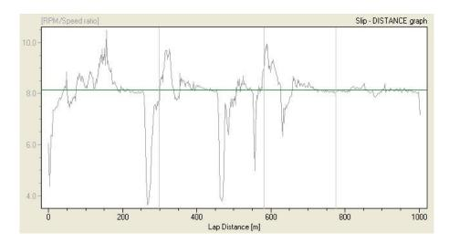
The Slip-Distance graph shows the gearing on the left axis and the lap distance in the bottom. The gearing is the green line. Everything above the line is the rear wheel spinning and everything below the line is the rear wheel slipping or sliding. You can use this graph to compare your driving style from lap to lap, and learn where it is efficient with an aggressive driving style and where it isn't. In order to make this graph you need a precise measurement of distance, speed and RPM.
