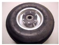
After the sensor disc is mounted, the centering bush is removed again. The wheel is now ready for mounting again.
