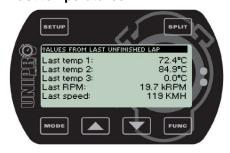
For all three temperature inputs, the temperature is stored at the split second when the engine stops. Therefore, if you have an engine crash you can see the three temperatures at that exact point in time when the engine stop and perhaps it will be clearer why it happened. Also the last RPM and the last speed is stored and shown on this screen.
