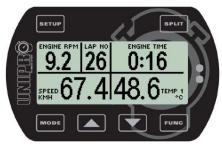
When the finish line is passed for the first time, the display change to show the engine stopwatch. This stopwatch is running all the time the engine is started. **No** lap times or delta times will be shown during the practice. However all data is stored as usual, and can be viewed in pit mode. The engine stopwatch will start from zero when the Laptimer is changed to pit mode and back again.
