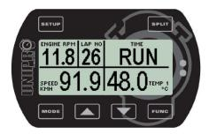
Time run mode is entered by pressing and holding while turning the Laptimer on with a short press on The display will show "RUN" in the display to indicate time run mode. This will be shown all the time in firstlap mode.
