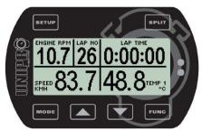
When the Laptimer is turned on with the button, it starts up in firstlap mode. This is the part of the race going from the pit to the finish line for the first time.
