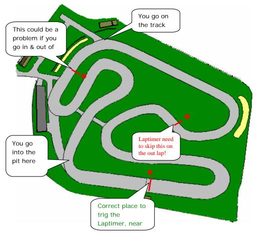
As you can see, there are three different magnet stripes on this track. It is very important to start (trig) the Laptimer near the finish line, in this example that is magnet number 2. That means that when you are driving out from the pit, the first magnet need to be skipped or you need to delay the trig by one magnet.
