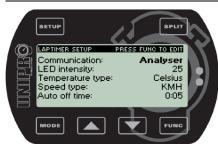
Typical connection to the outside is either IrDA (infrared) or USB. If you set the Laptimer to use IrDA, it will go to PC mode after leaving pit mode. If it is set to use USB, it changes directly to PC mode when the USB cable is connected.
