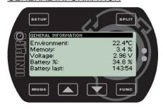
Here you can see information about environment temperature, memory usage, battery voltage, battery status and battery lifetime. This screen is showing a real time view of these values.
