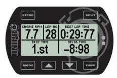
When the Laptimer is passing the finish line, it is showing the difference between the current lap and the best lap and its position. In the shown example, the current lap is 8.98 seconds better than the previous best lap and the current lap is the best lap (in position 1) This information is shown for 5 seconds before changing back to data display. Only times between +/- 9.99 seconds and positions from the 1st to 10th are shown
