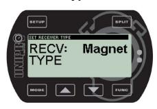
The Unipro Laptimer can use all types of receivers. You can choose between IR (infrared), Loop (AMB active loop) and magnet (magnet stripe in the track).
