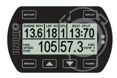
When driving with splits, everything is stored on splits as well as laps. Use the button to toggle between all the splits stored in the Laptimer. This example shows the maximum data and the split time for split number 1.
