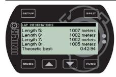
You can view the lap length for each lap stored in the Laptimer. In the same screen, you can see the calculated theoretical best lap time, which is the time you get when all the best split times is added to make one theoretical lap. Use the and buttons to select the lap you want to view.
