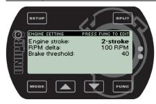
You can set the engine stroke between 1 and 8. RPM delta is the number of engine revolutions you want to have in the intervals if you use the shift light function. In this screen you can also set the number of magnets on the speed sensor disc to a different number than 6, which is the standard number of magnets on the Unipro sensor disc. Use and abuttons to find the setting you want to change. Use
