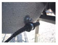
The Loop receiver is mounted parallel with the seat and needs to point backwards against the rear axle. Make sure, that nothing comes between the receiver and the track.
