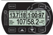
Pit mode is for analysing the data stored in the Laptimer. If is pressed from either firstlap mode or running mode, you will enter pit mode.
