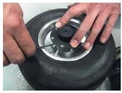
The sensor disc is placed over the centering bush and it is held firmly down. Then tighten the three small screws that fixes the sensor disc to the wheel. Tighten the three screws hard, so the sensor disc doesn't go loose when you're driving.
