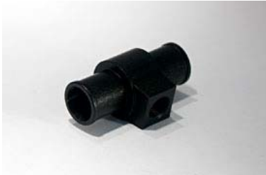
This is the T-junction used for the water sensor.
