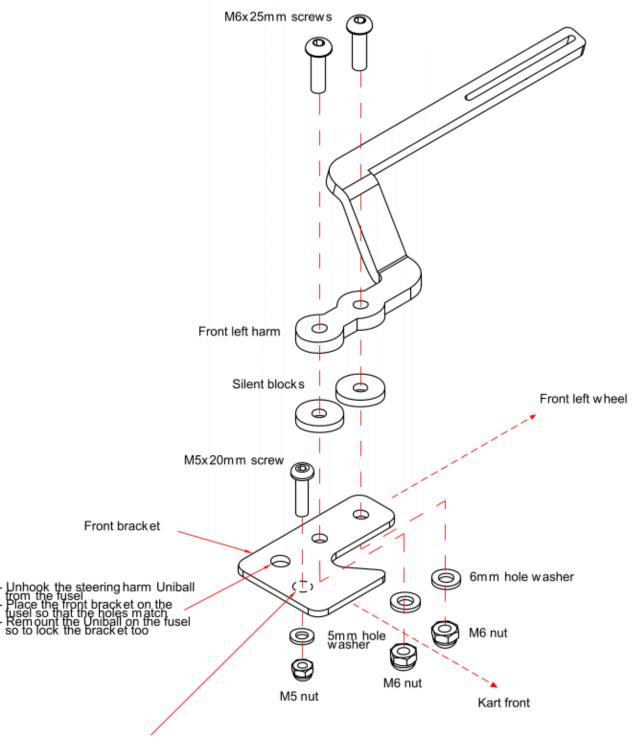
Drill (5mm diameter) the front bracket according to the fusel geometry
