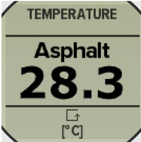
The first screen in the sequence is the asphalt temperature.
