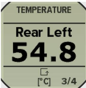
Large current temperature for Rear Left tire, an arrow to show the sequence direction and numbers in the corner showing that you are measuring tire 3 of 4.
